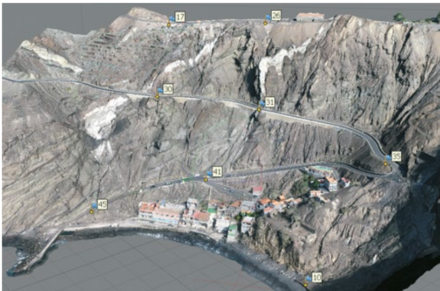
Figure 1. Digital terrain model produced from drone photogrammetry.
