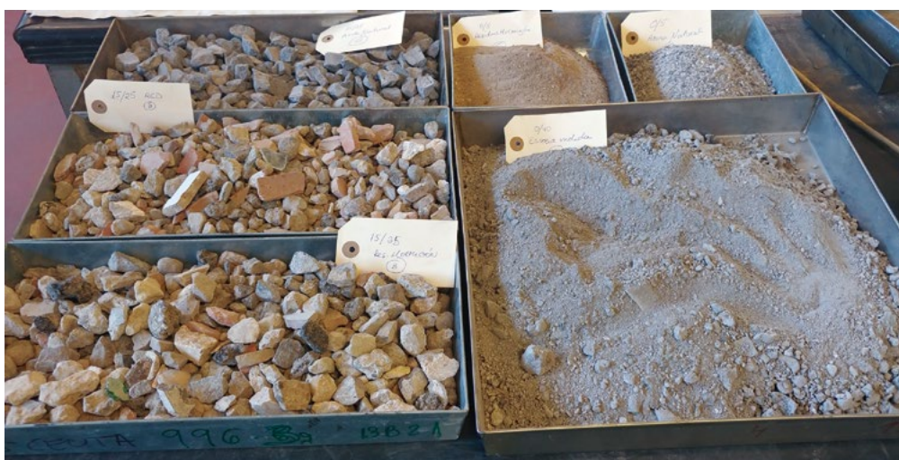
CDW aggregates and USW incineration slags for concrete production.
