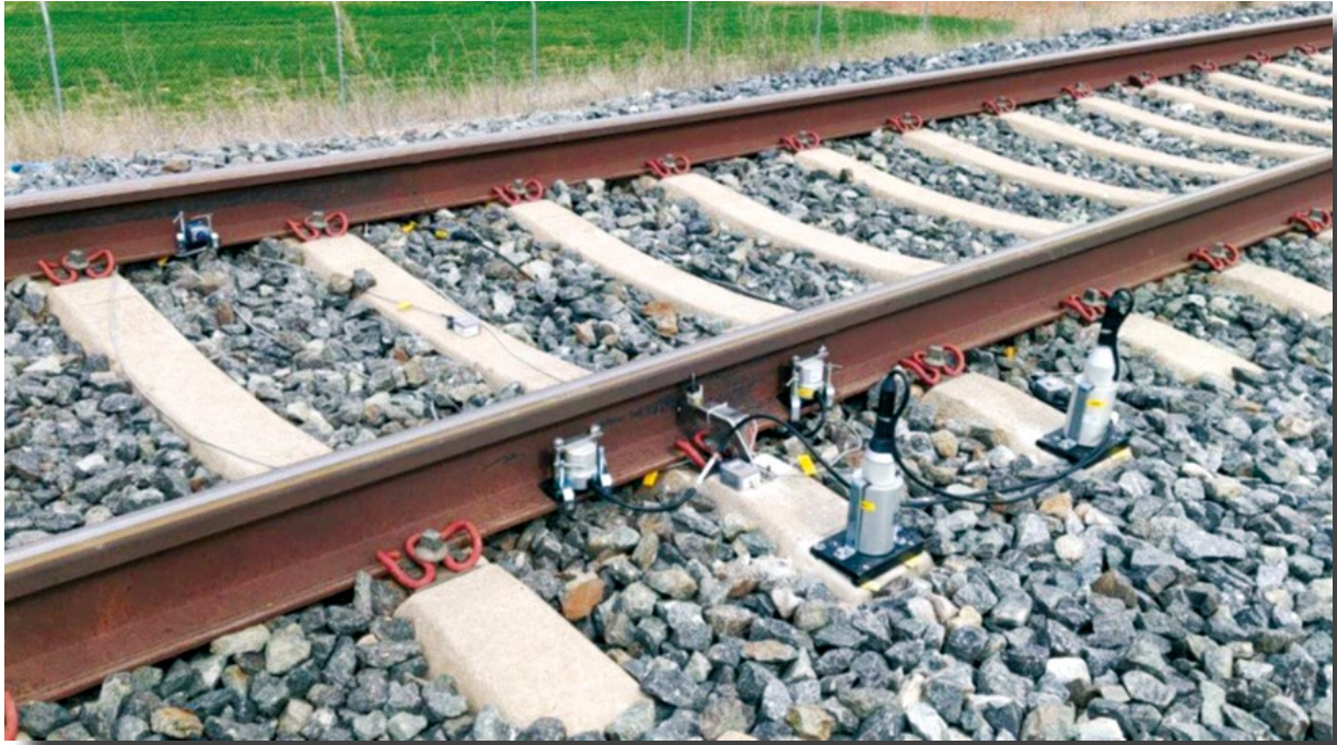
Figure 4. View of the instrumentation mounted on a section of the Madrid-Barcelona high-speed line.
