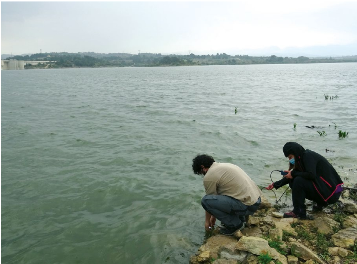
Measurement of unstable parameters in a water sampling campaign for isotopic study of water tightness of the Bellús reservoir.
