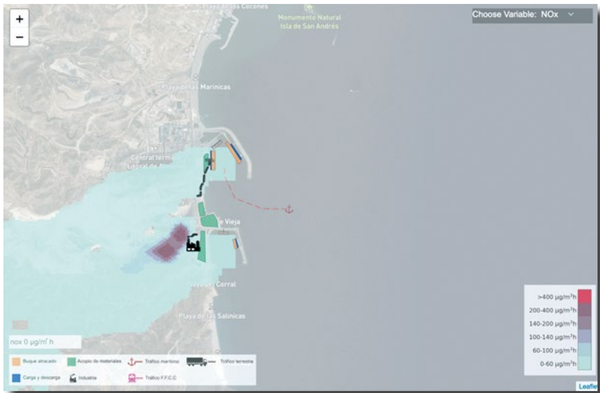
Simulation of dispersion of pollutants (NOx) in one day of operation.
