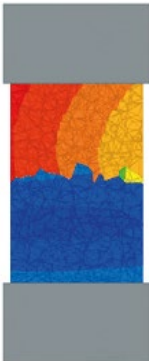
Numerical simulation of direct tensile fracture of a rock sample.
