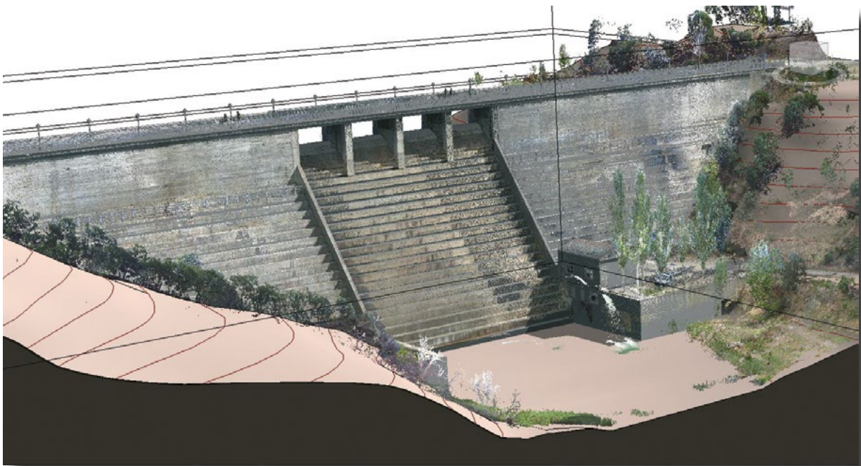
General view of the virtual model, overlaying the 3D point cloud and the BIM model.
