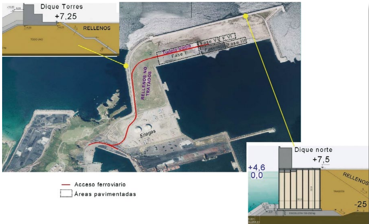
Layout of the railway access to the north quay of the port of Gijón and dock sections.
