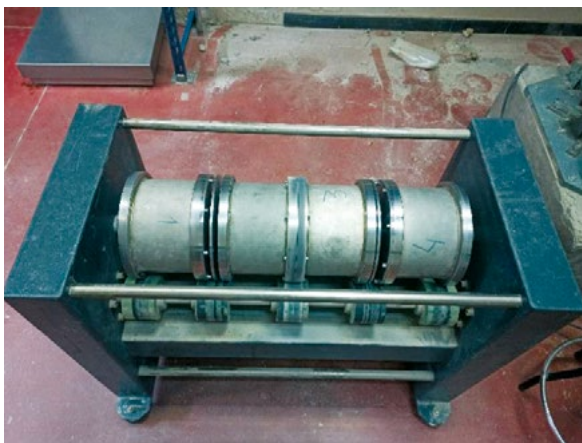
Figure 3. LG-CEDEX Micro Deval equipment used for ballast degradation studies.
