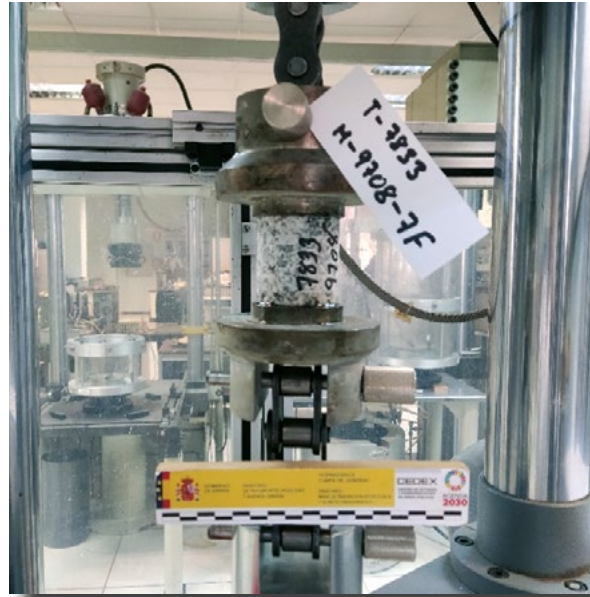
Direct tensile test on a low slenderness granite specimen.
