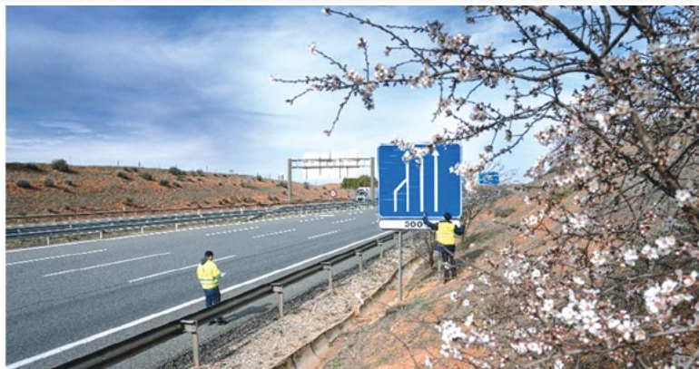
Activities of LCEYM's Area of Materials: Study of the concrete of the Tentudía dam (Badajoz) (above left), inspection of La Cruz Santa reservoir (Tenerife) (above right), and measurement of the retroreflection of vertical signage (below).
