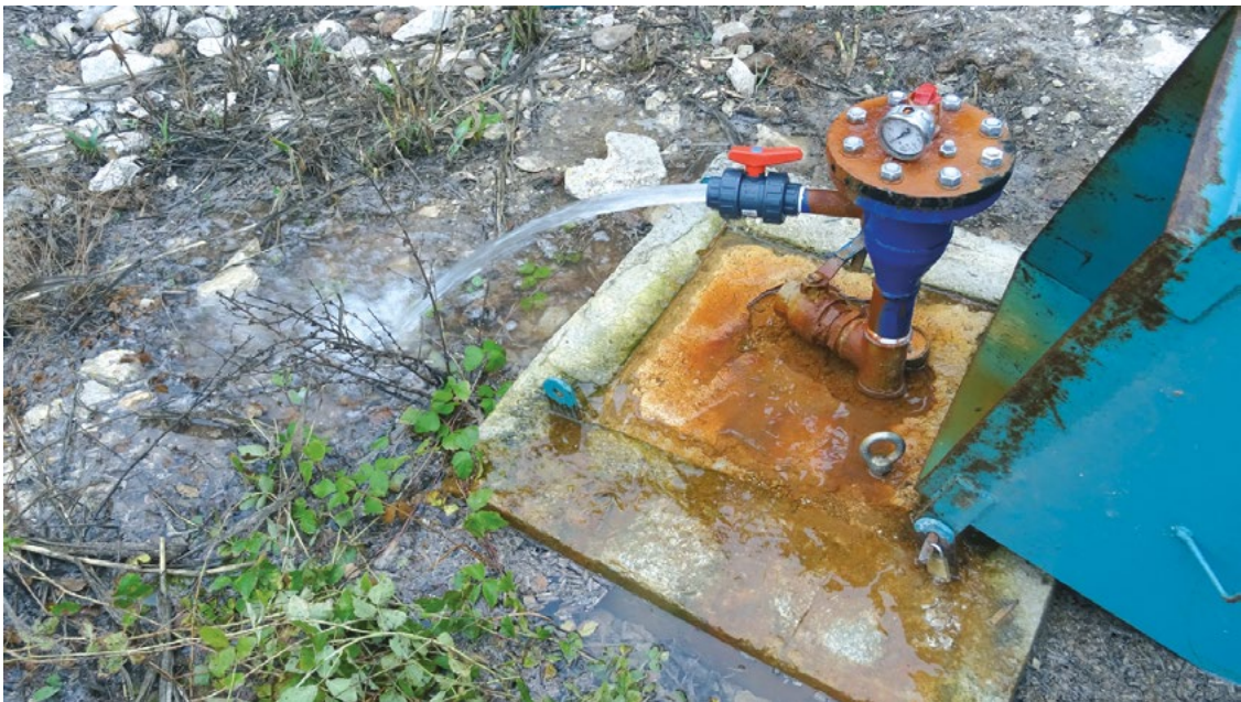
Upwelling borehole used as a piezometer and sampling point located in an aquifer downstream of the Bellús reservoir.
