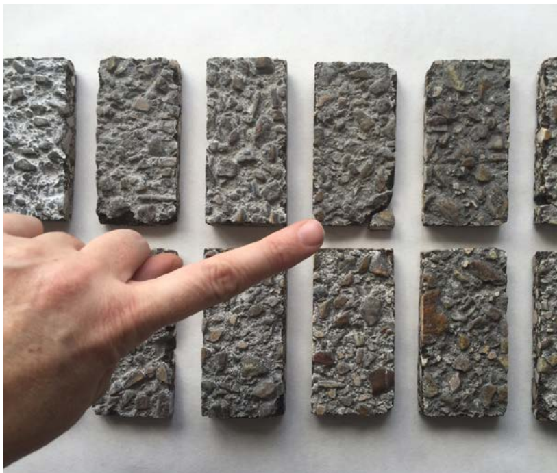
Bituminous mixture test specimens from the Paseo de la Chopera after different exposure times to traffic
