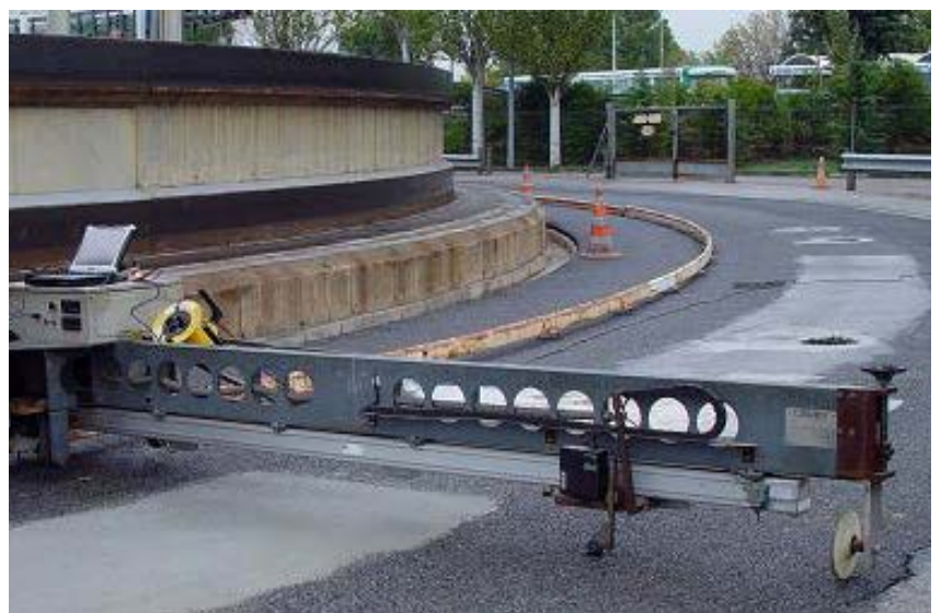
Transverse evenness measurement on a test track
