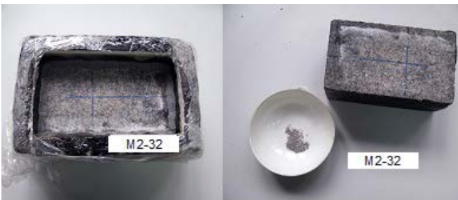
Frost resistance test
