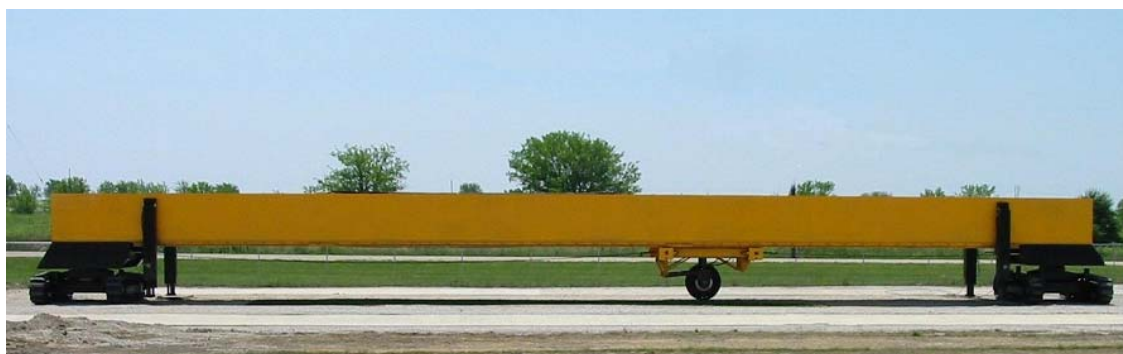
FIGURE 7 Advanced Transportation Loading ASsembly (ATLAS).
