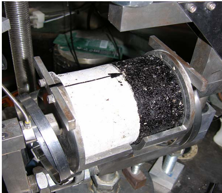
FIGURE 2 HMA-PCC specimen ready for testing.
