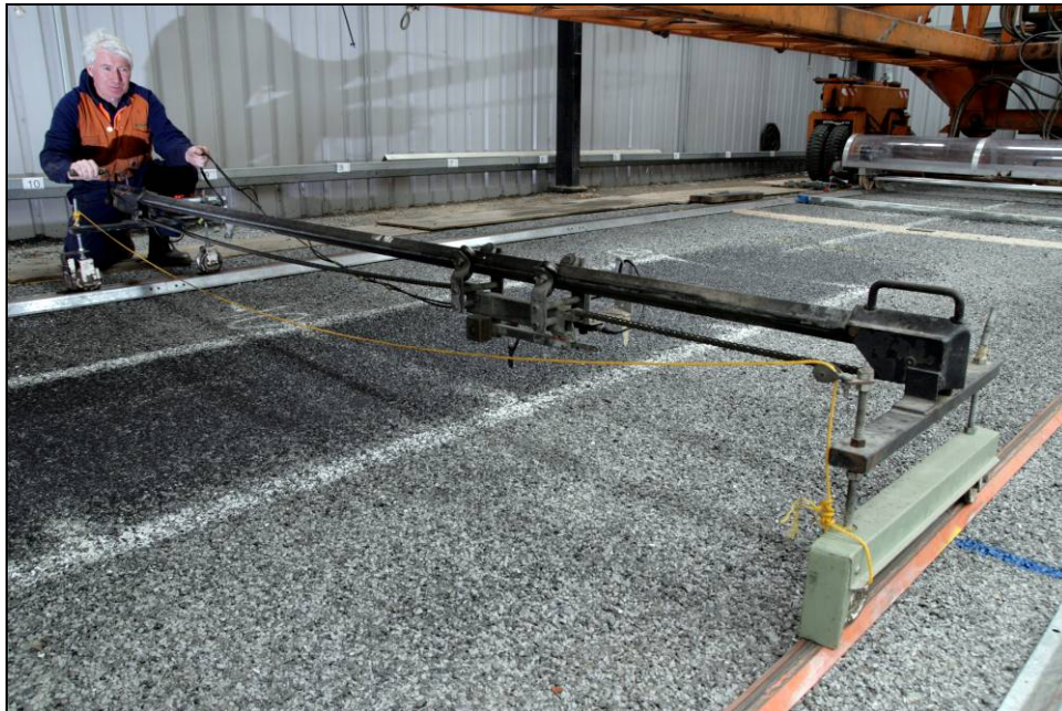
FIGURE 3 Transverse profile measurement of test section under ALF
