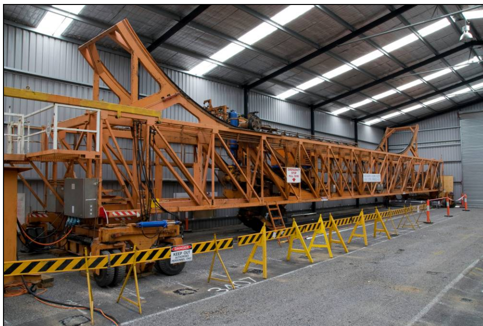
FIGURE 1 Accelerated Loading Facility operating inside shed
