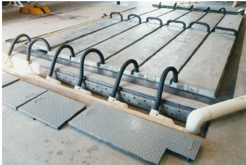
Figure 5. Surface Heat Exchangers
