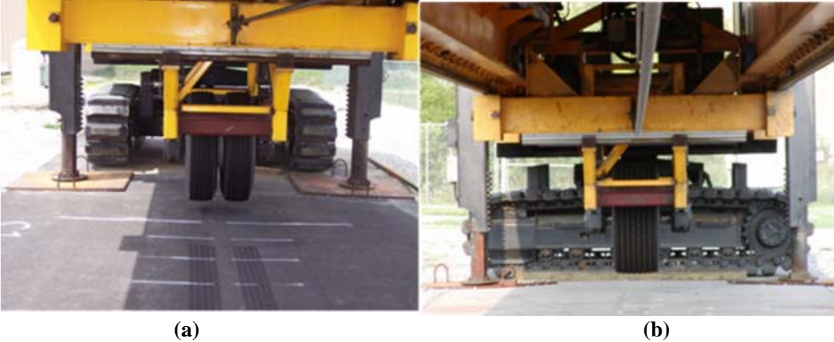
FIGURE 2 Advanced Transportation Loading ASsembly (ATLAS) with (a) dual-tire assembly; and (b) wide-base tire.
