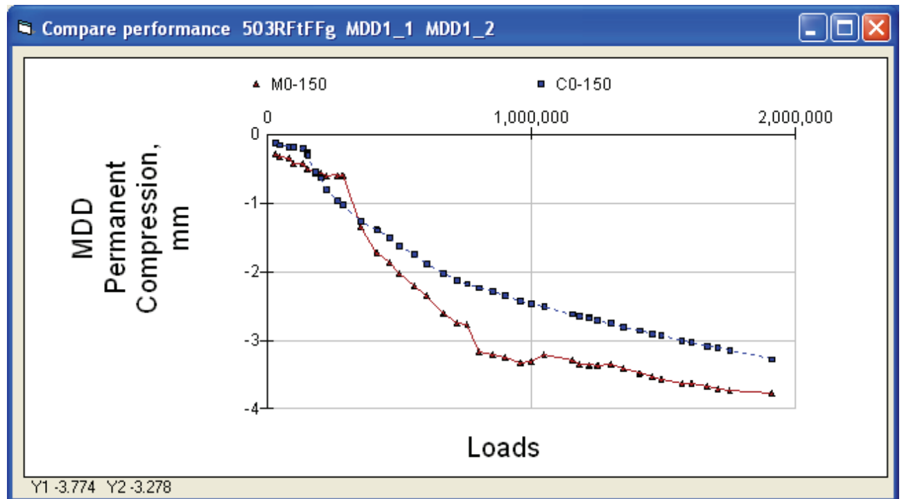
Figure 4. Permanent deformation of the asphalt layers, measured and calculated.
