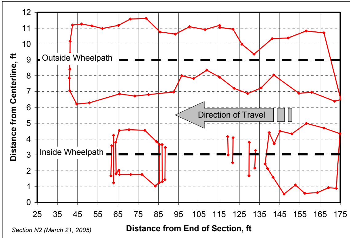
FIGURE 3 Example of Crack Mapping.
