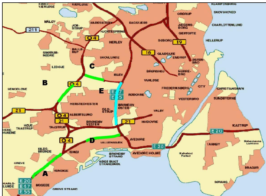
Figure 1 Location of reference motorway sections around Copenhagen with cement bound base. Blue: Reflective cracking. Green: No reflective cracking.
