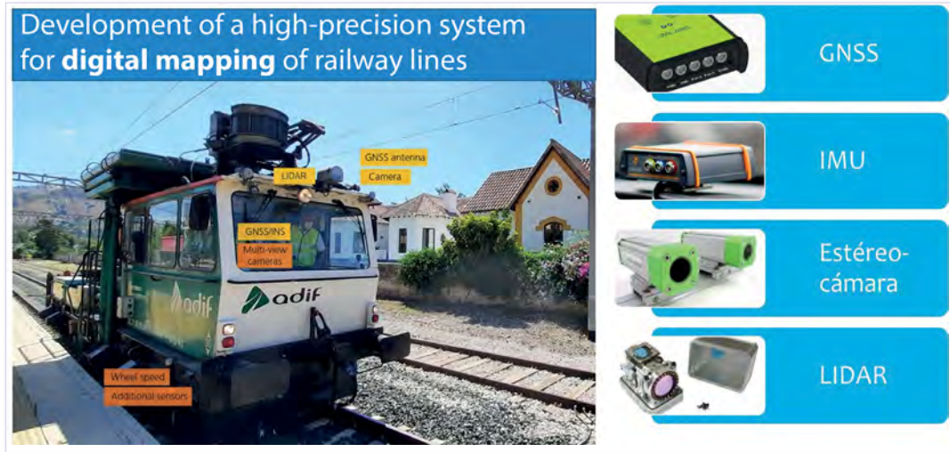
Equipment of an Adif railcar for the European project RAILGAP (financed by the EUSPA).
