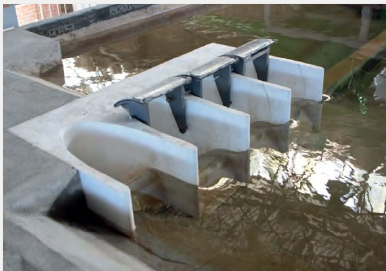
↑ Physical modelling of the new spillway of the Yesa dam (Ebro RBA).
