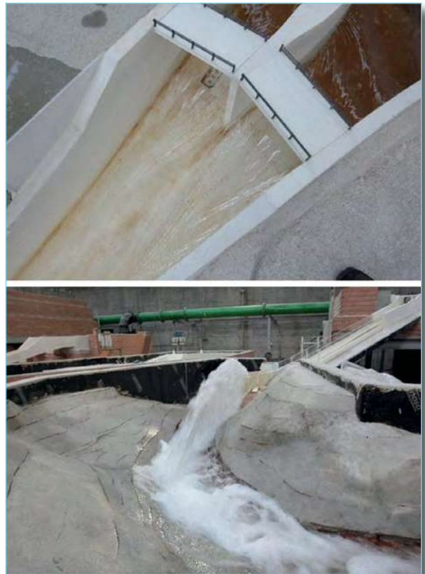
Upstream structure and spillway of the physical model of the Arenós dam.
