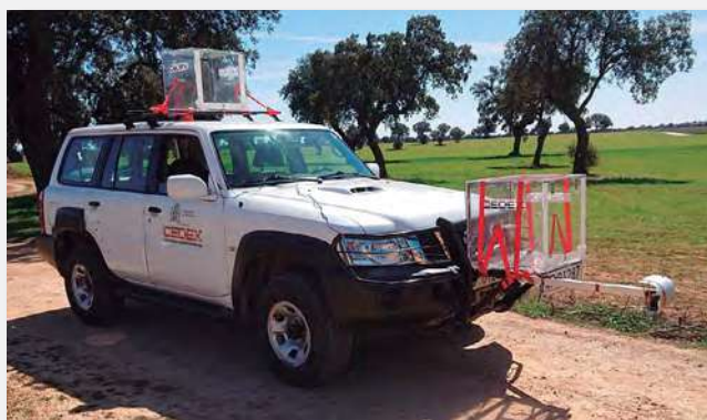
← Installation of two collectors at different levels for 2 and 3. A webcam has been installed at the front end for recording the tests.
