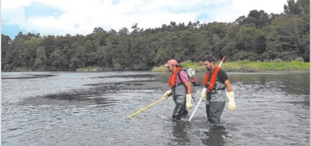
Sampling of ichthyological fauna with portable electric fishing equipment in the Miño River for the Albufeira Project (2020).
