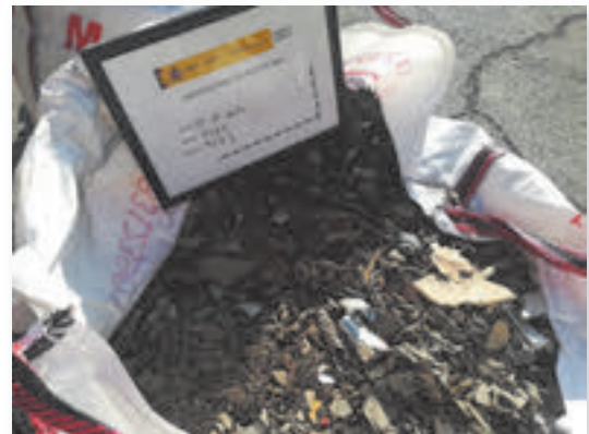
Figure 9. Sample of material from a non-hazardous waste landfill for testing in the 1 x 1m direct shear box.
