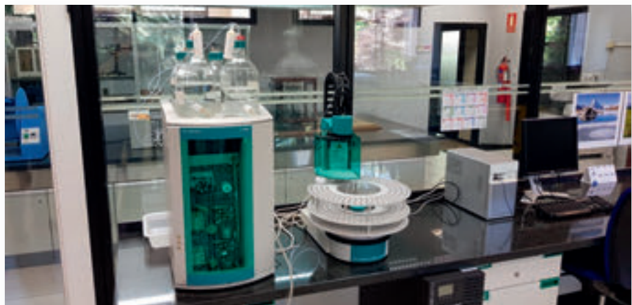
Figure 10. IC ion chromatography equipment of the chemistry section of the Laboratorio de Geotecnia.
