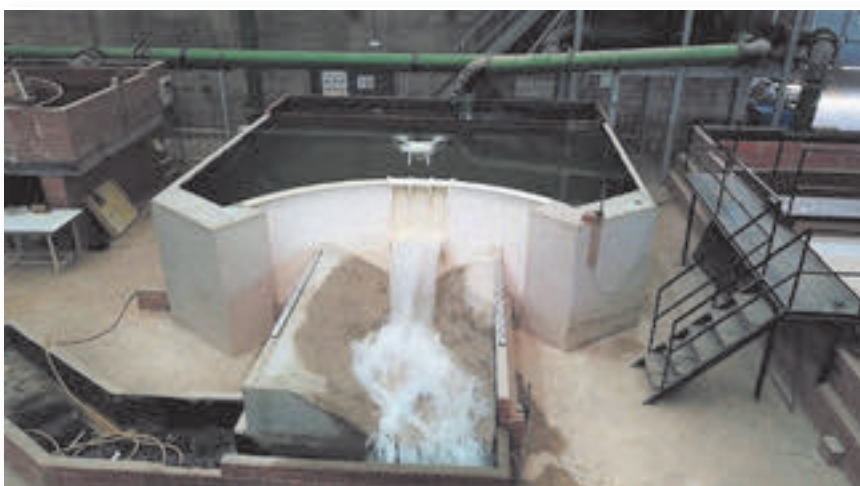
Operation of drone equipment during physical modelling tests.
