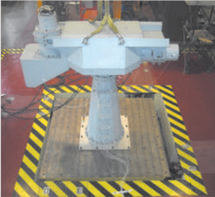
Vibration and shock test on a BPE-PAR Stabilizer.
