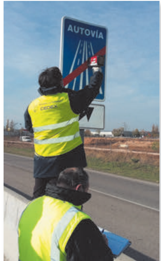
Measuring retroreflection of vertical signals in highway A-4 section 3.
