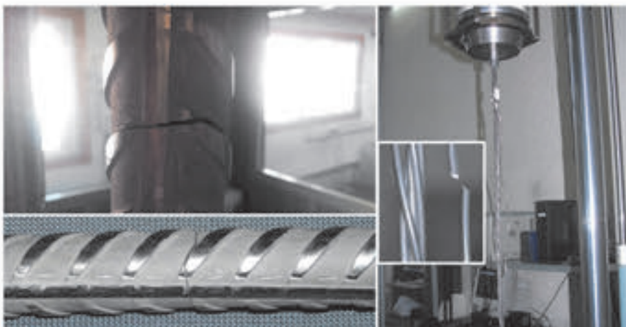
Steel reinforcement of concrete fractures.
