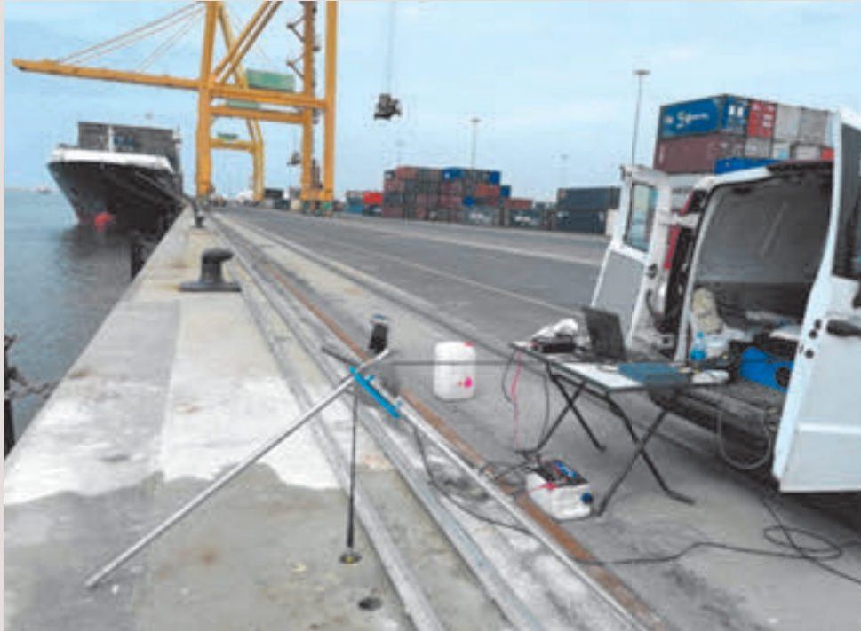
Measurement system with the probe inserted in a borehole.
