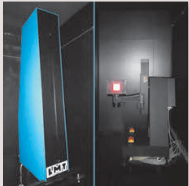
View of the retroreflectometer and goniometer.
