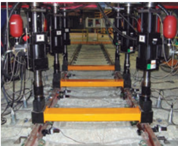
Detail of three pairs of servo-hydraulic actuators.
