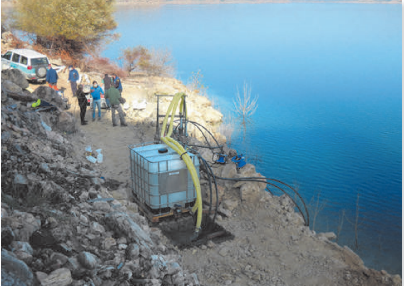
Figure 6. Large-scale permeability test (Alcorlo dam, upstream slope).
