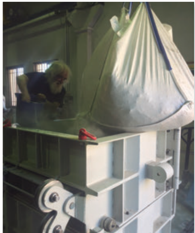
Sample placed by vertical discharge.
