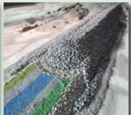
Figure 6. Expansion of the port of Aberdeen (UK). Physical model test. Final and construction stages.
