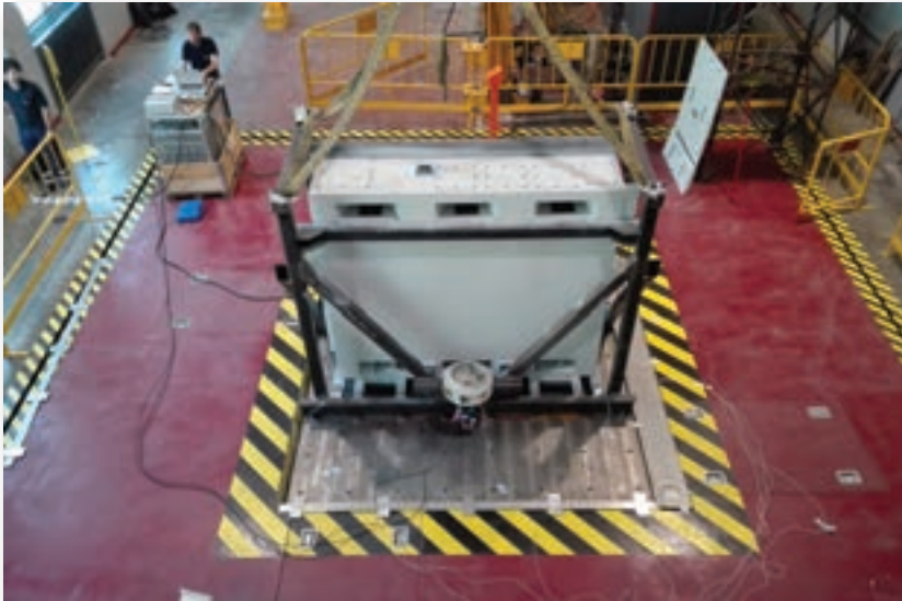
Vibration and shock test on a converter equipment.
