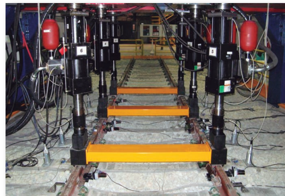
Detail of sensors in the railway track.
