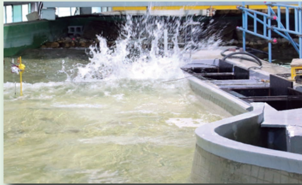
Figure 3. The Sardinero beach (Santander). Study in numerical (SPH) and physical models (E: 1/10), for the overtopping reduction on the seafront (avda. M. G a Lago).
