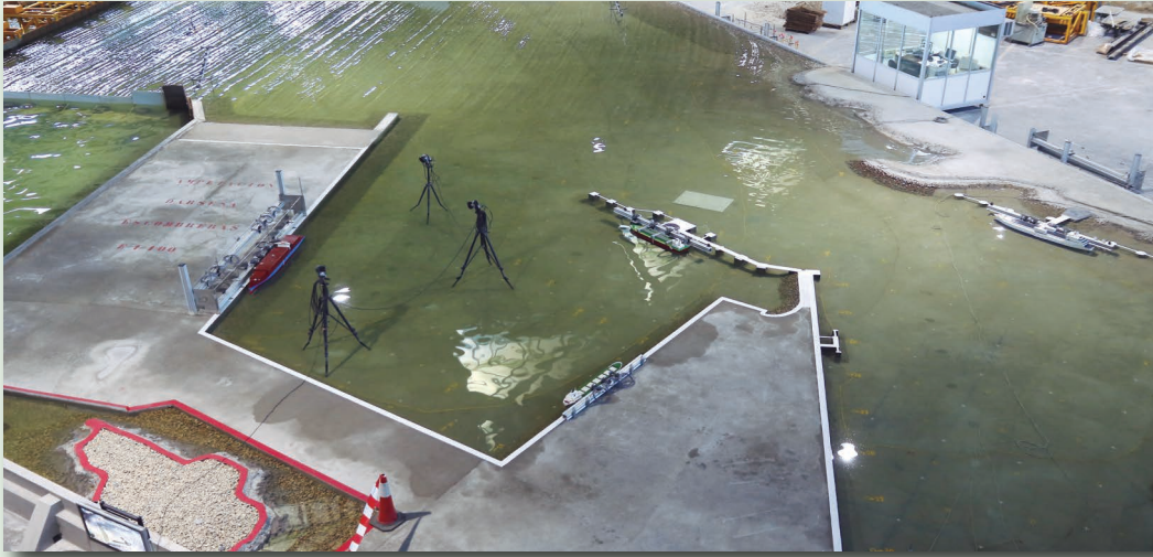
Figure 2. Three-dimensional physical model of agitation and moored ships for the study of the extension of the Escombreras dock (Cartagena).
