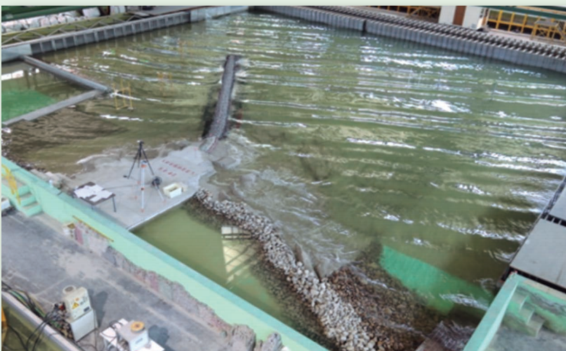
Figure 6. Expansion of the port of Aberdeen (UK). Physical model test. Final and construction stages.
