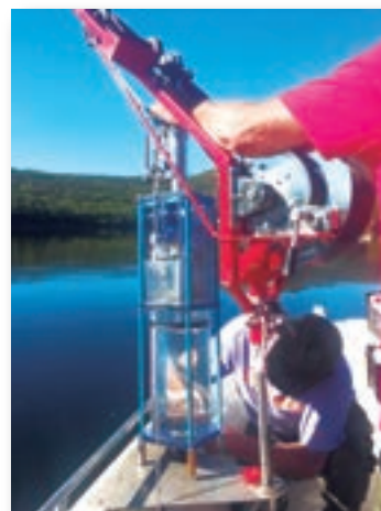
Above. Obtaining sediment cores in a frozen lake with piston running and percussion on a platform.
