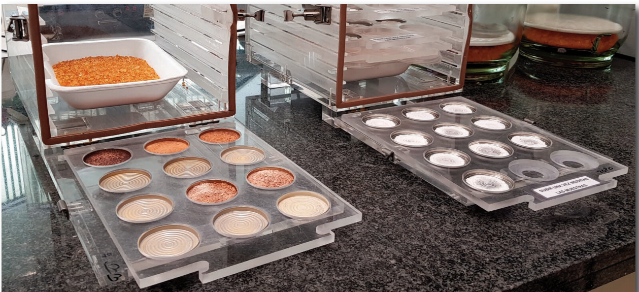
Planchettes for measuring radiological indices in continental (left) and marine (right) water.
