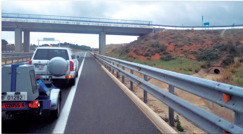
CEDEX FWD checking the bearing capacity in a road section.
