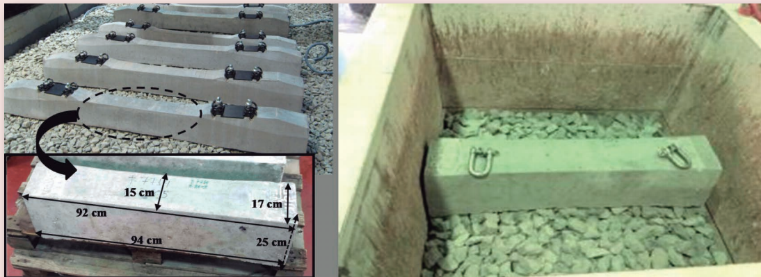
Figure 4. Geotechnical characterization of the sleeper-ballast contact.
