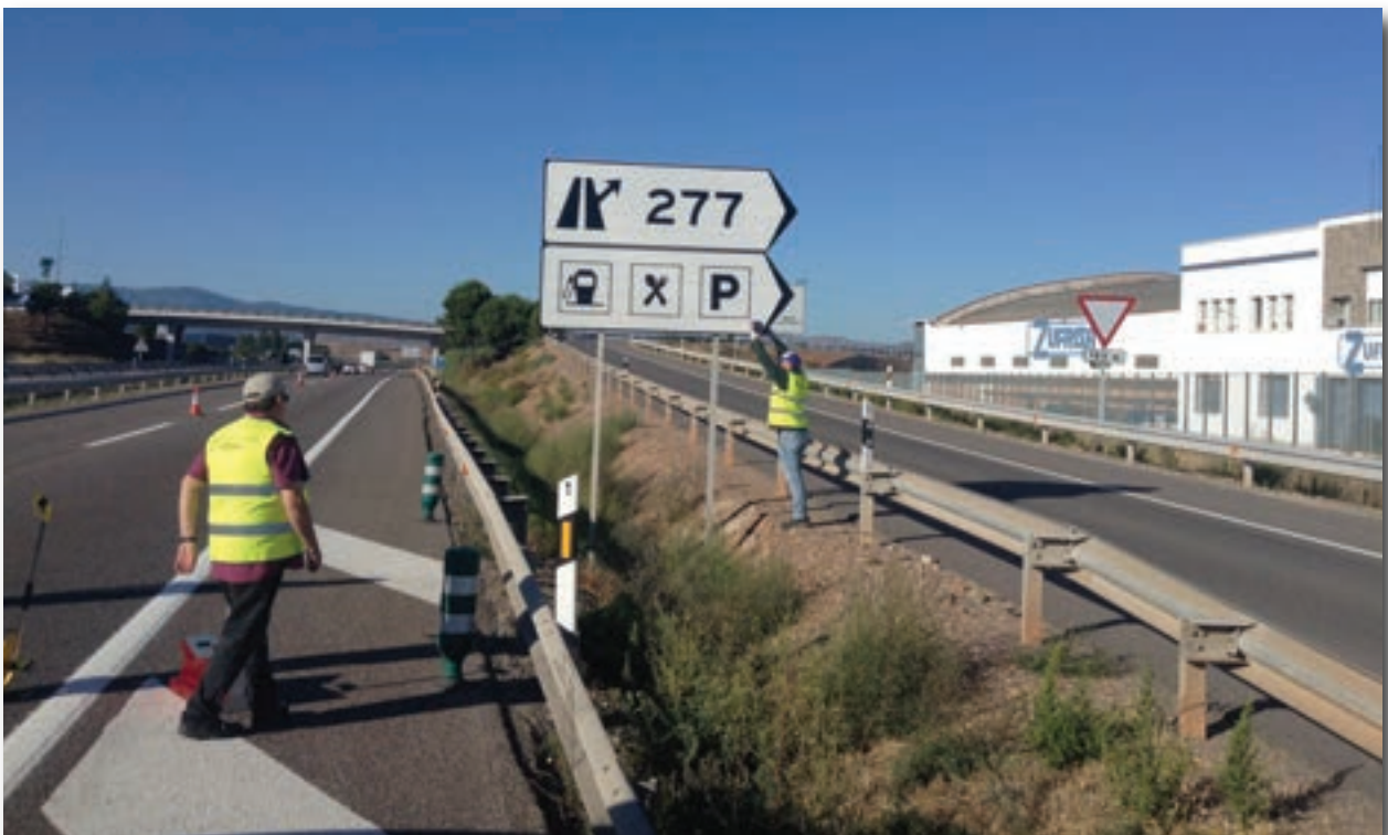
Measuring retroreflection of vertical signals in highway A2, section 4.
